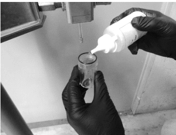
6 – Use only the oil supplied by Fillon Technologies. Fill up to the maximum oil level.
