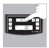
If a different value is displayed: Tare the scale using the [+0/16] key (Zero/Tare).
