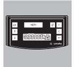
Once the scale has been turned on, it will run an automatic self-test. This ends when the display shows 0.0 g.
